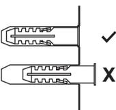
⚠ Anchors can be just used for concrete wall , not for wood or stud.
